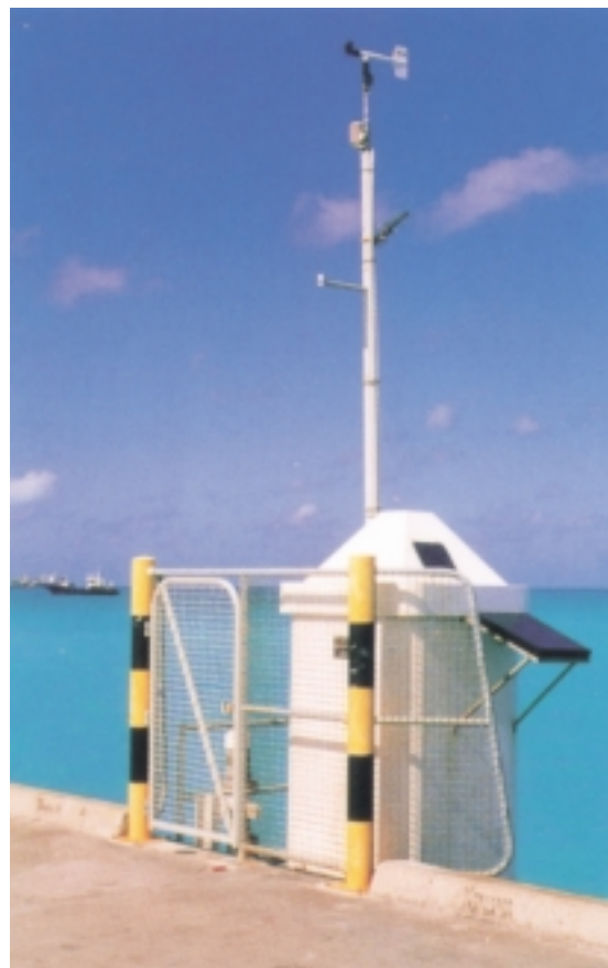
The SEAFRAME station of the South Pacific Sea Level and Climate Monitoring Project, established at eleven sites in the Pacific.
